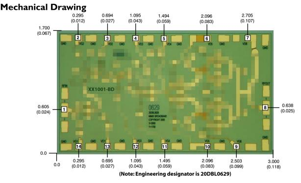
Units: millimeters (inches) Bond pad dimensions are shown to center of bond pad. Thickness: 0.110 +/- 0.010 (0.0043 +/- 0.0004), Backside is ground, Bond Pad/Backside Metallization: Gold All DC Bond Pads are 0.100 x 0.100 (0.004 x 0.004). All RF Bond Pads are 0.100 x 0.200 (0.004 x 0.008) Bond pad centers are approximately 0.109 (0.004) from the edge of the chip. Dicing tolerance: +/- 0.005 (+/- 0.0002). Approximate weight: 3.987 mg.
